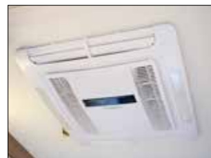
AC Dometic Fresh Jet FJX72600, FJX4 2200 i enkelte mindre modeller (standard Imperial)
